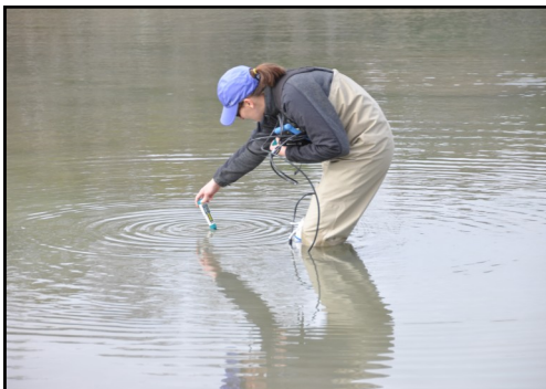
Dr. Seldomridge takes a measurement of the dissolved oxygen level in the North Llano River.
