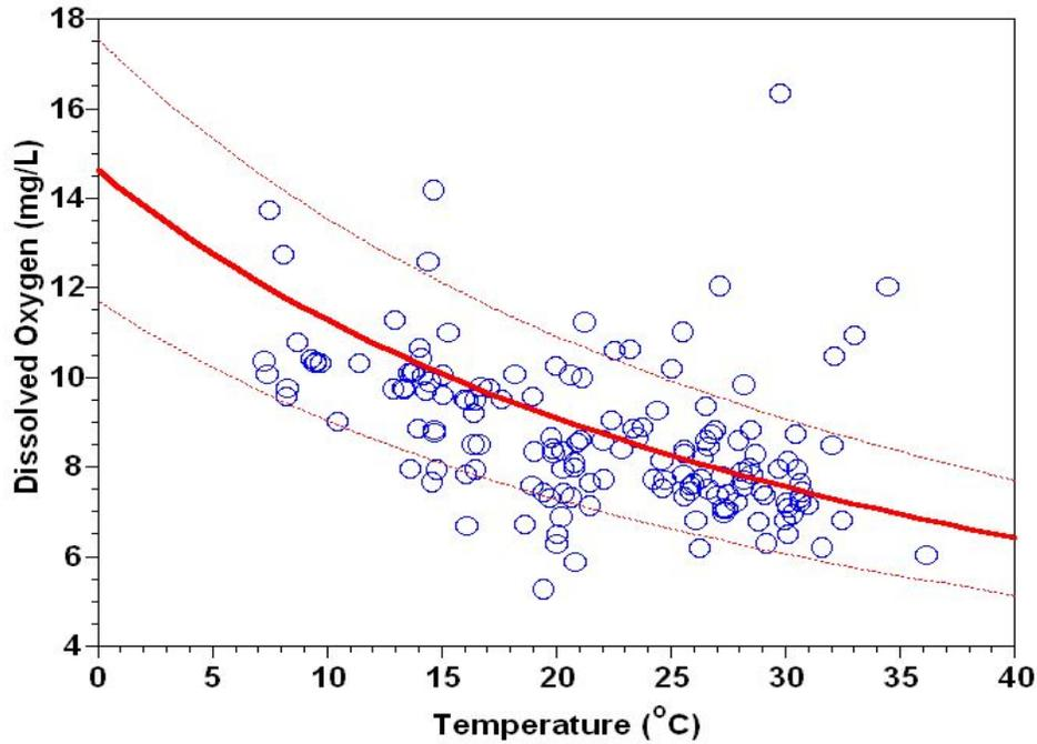
Figure 3. Dissolved oxygen and water temperature from all monitoring stations. The solid line represents 100% saturation, and the upper and lower dashed lines represent 120 and 80% saturation, respectively.
