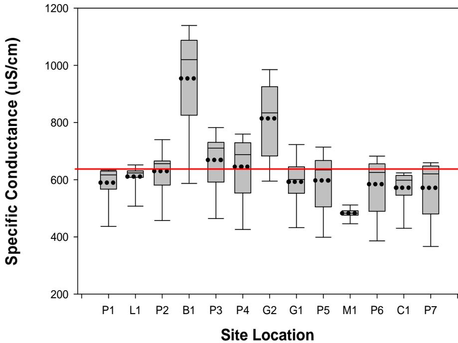
Figure 2. Box-plot diagrams of specific conductance (uS/cm) by site location. The red line represents the grand mean.
