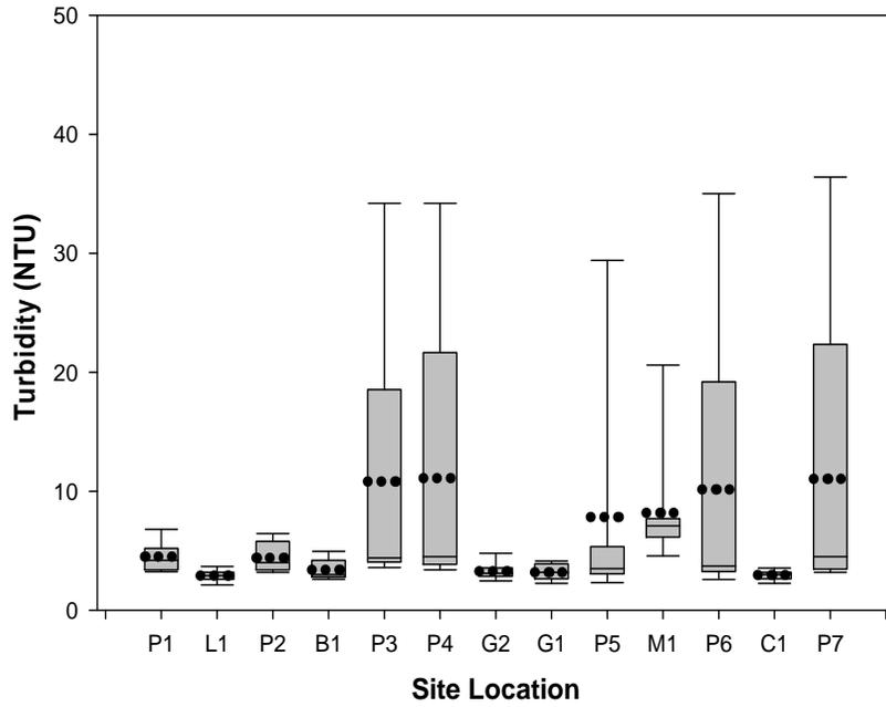
Figure 4.1. Box-plot diagrams of turbidity (NTU) from all monitoring stations.
